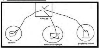
It is just another name of the same exact file. We can create hard link file by using In command, In originalfile hardlinkfile
