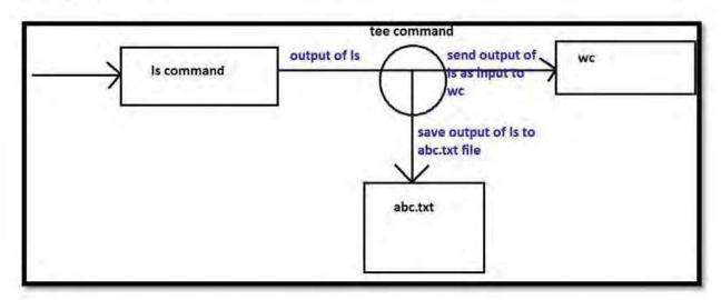
Eg 2: To save the output of Is command to a file and send that output as input to wo command
