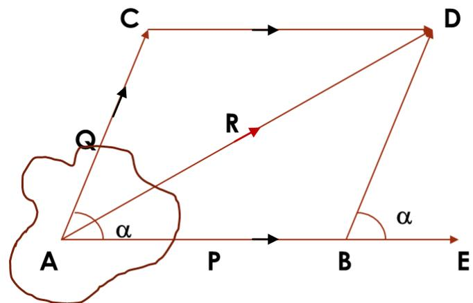
$\vec{AB}$ ,  $\vec{AC}$  are components  $\vec{P}$ ,  $\vec{Q}$  are constructing parallelogram ABCD as shown in Figure.
