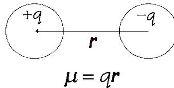
*Fig. 1.1: Electric dipole*
