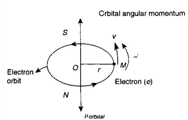
Fig.2.1 Revolving electron in an atom produces magnetic moment
