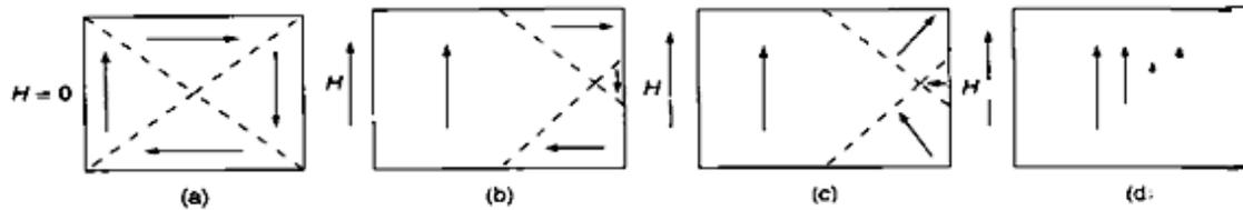
Fig. 2.6 (a) Domain orientation in the absence of the magnetic field (b) Domain enhancement shrinkage due to weak fields (c) Domain rotation due to strong fields (d) Saturation due to very high fields
