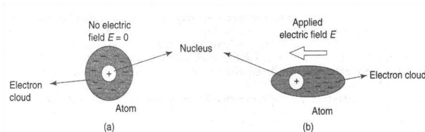
Fig. 1.8. (a) Un polarized atom in the absence of field
