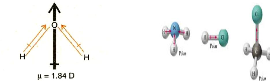
Fig.1.3: Polar molecules with net dipole moment ( $\mu \neq 0$ )
