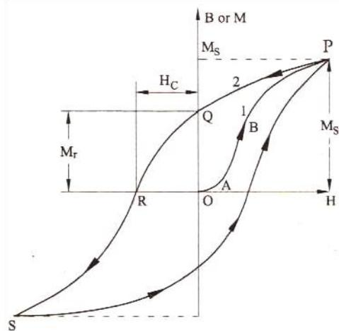
Fig. 2.7: Magnetic Hysteresis curve (or)  $B - H$  curves of a Ferro magnetic material
