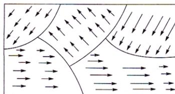
Fig. 25.5: Different possible orientations of domains
