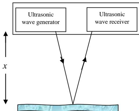
Figure 4.3. Measuring depth of sea using SONAR
