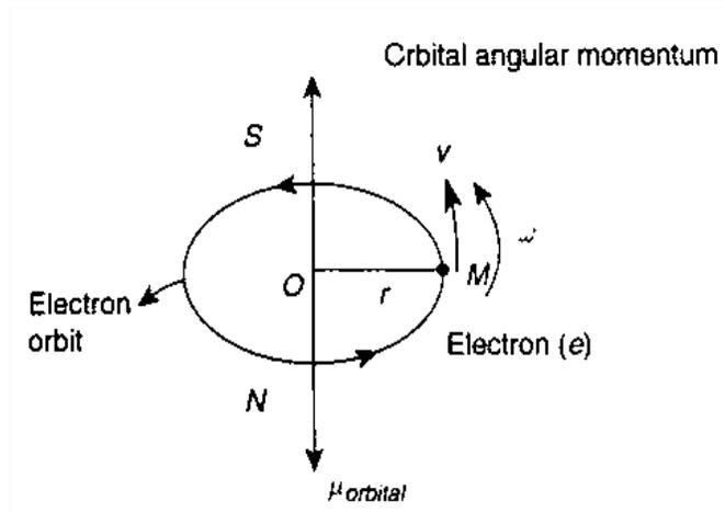
Fig. 2.2 Orbital magnetic moment of electrons
