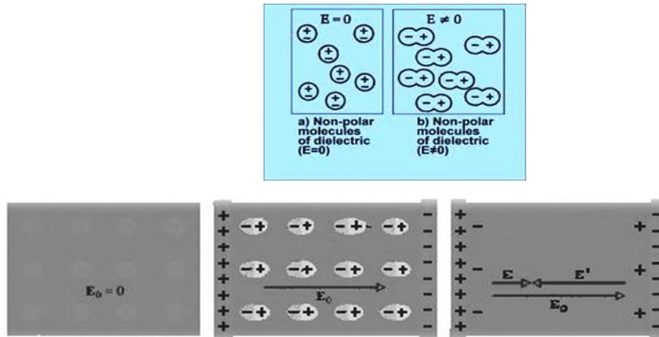
Fig. 1.5: (a) non polar dielectric in  $E=0$  (b) Non polar dielectric when 'E' is applied (c) Totally polarized non polar dielectric with net field
