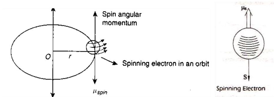
Fig. 2.4 Spin magnetic moment of electrons
