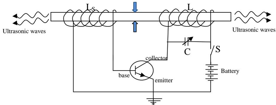
Figure 4.1. Magnetostriction oscillator
