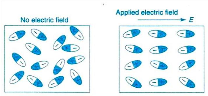
Fig. 1.10: Orientational polarization
